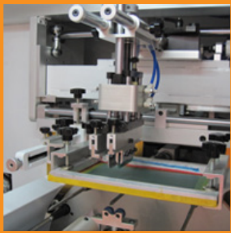
Close-up of print head with X/Y/R adjustment
